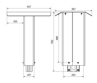
Next Green Polebox is a post mount for charging boxes for mounting on a 60 mm pipe post. Polebox makes it easy, for example when changing from engine heater location to charging location and can therefore be used to replace an engine heater hood. The product is intended for feeding electrical cables inside the pole tube.
