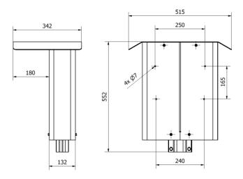
such as a Wi-Fi-router or a 3G/4G modem or power supply. Everything fits neatly inside the box. Polebox is made of Swedish steel and powder coated to provide the highest quality.
