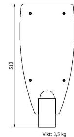
Poleplate charging box holder is a cost-effective pole mount. Poleplate 225 Z facilitates changing an engine heater station to a charging station and can be used to replace an engine heater central.
