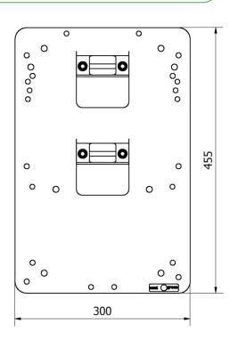
$Next\,Green\,Pole plate\,300\,Ceiling\,is\,a\,pole\,tube\,bracket\,for$ charging boxes, intended for ceiling mounting on 60 mm pole tube. Poleplate is made of steel. Poleplate is designed to easily mount a charging box.
