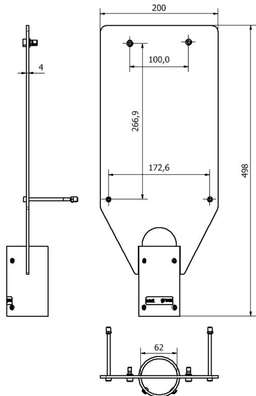
**Next Green Poleplate 200 A** is a EV-charger mount for installation on a  $\varnothing$  60 mm tube or pole. Poleplate is made of Swedish steel and powder coated to provide the highest durability and quality. Poleplate enables easy mounting of a charging box to a steel tube or pole.
